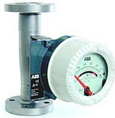
Figure 5. Variable-area flowmeters typically contain a float that is forced upward by the fluid passing through. The point of equilibrium between this force and that of gravity indicates the volumetric flow rate. (Photo courtesy of ABB Inc. )
