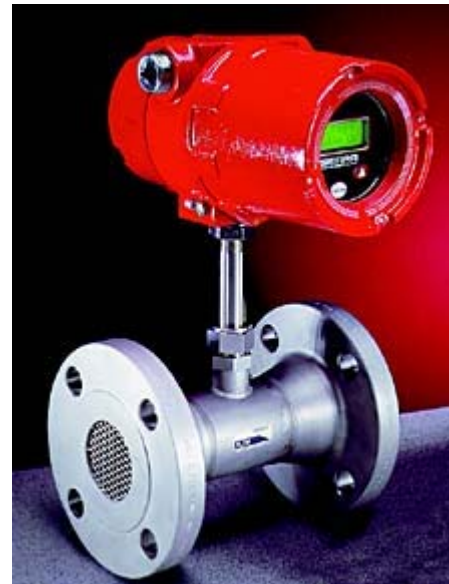
Figure 11. Thermal flowmeters measure mass flow directly. Some of these devices put heat into the flow stream and measure how long it takes to dissipate; others measure the amount of energy required to maintain a constant temperature in the stream. They are used for low flows, primarily gas. (Photo courtesy of Sierra Instruments )
