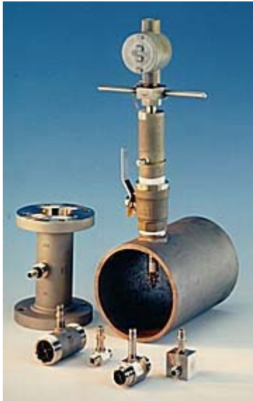
Figure 3. The rotor in turbine flowmeters spins at a rate proportional to liquid flow rate. Shown here are an insertion (center) and an inline type (left). The small meters in the foreground are also turbines. (Photo courtesy of Hoffer Flow Controls Inc. )
