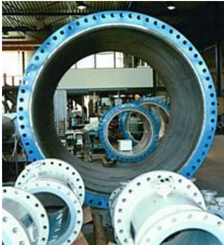
Figure 7. Magnetic flowmeters operate on Faraday's law of electromagnetic induction and therefore work only with conductive liquids. A current applied to coils mounted on or outside the flow pipe generates a magnetic field inside the pipe. The liquid passing through generates a voltage proportional to flow rate, which is detected by electrodes on either side of the pipe. (Photo by Flow Research , courtesy of Krohne)
