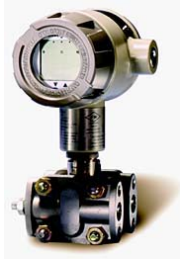
Figure 1. Differential pressure flowmeters insert an obstruction in the flowstream to reduce the flow rate and thus the pressure. Flow rate is calculated by taking the difference between upstream and downstream pressures. (Photo courtesy of Honeywell )
