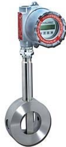
Figure 9. Vortex flowmeters measure flow by placing a bluff body across the stream. Flow rate is calculated by multiplying the pipe area by the flow velocity, which is proportional to the frequency of the vortices generated by the bluff body. These devices are used with liquid, gas, and steam. (Photo courtesy of Venture Measurement Co. )
