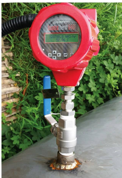
Figure 2. Close-up of thermal mass flowmeter, part of Sierra Instruments' Big-3 for flow energy applications
