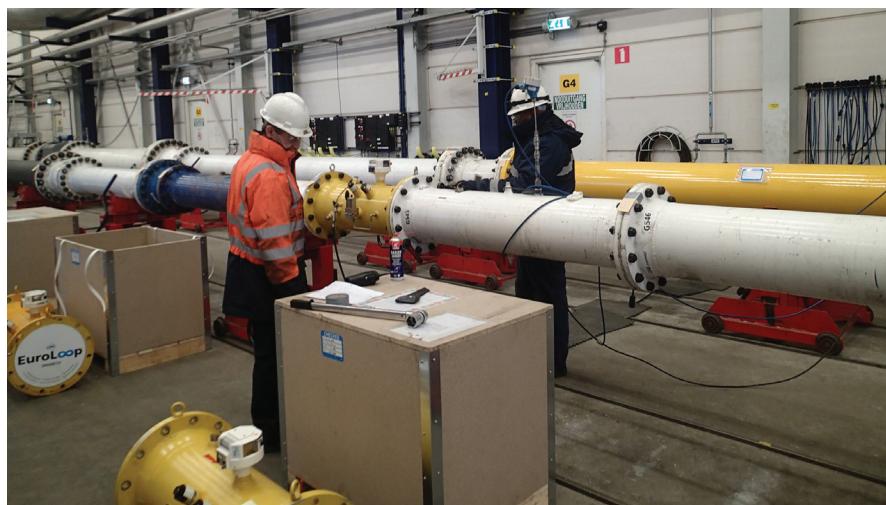
An ultrasonic flowmeter gets placed in a test stand at NMi Euroloop.
