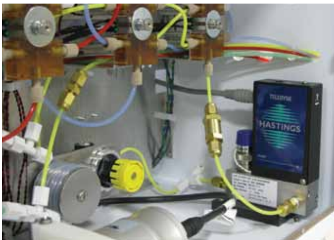
Mass Flow Controllers are used in a wide variety of OEM analytical systems. The analytical instrument shown here is designed to accurately detect carbon content in aqueous matrices down to the PPB level using a high temperature combustion furnace and a pressurized NDIR detector. (Photo courtesy of Teledyne Hastings)
