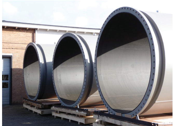
One of the advantages of magmeters is their ability to support large line water & wastewater applications at a reasonable price point. (Photo courtesy of KROHNE.)
