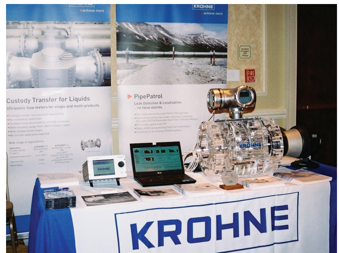
KROHNE's Altosonic V12 is a custody-transfer gas flowmeter that has 12 chords. Here is a transparent version of the meter on display at the 2012 CEESI Ultrasonic Flowmeter Workshop to show its inner workings.
