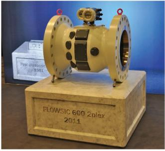
Ultrasonic flowmeters, along with Coriolis and multiphase, are among the most popular technology focal points at flow measurement conferences today. This is primarily due to their suitability for critical oil and gas custody-transfer applications.
