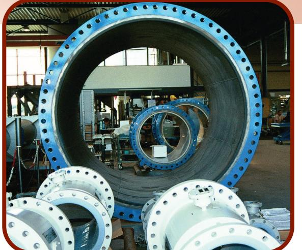
Magnetic flowmeters can support a wide range of pipe sizes.
