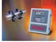
The DigitalFlow GC868 clamp-on ultrasonic flowmeter measures gas flow at high or low pressures. It works on up to 36-in. pipes made of any material. Accuracy is 2% of reading with repeatability within 0.5% of reading. No tapping or cutting of the pipe is required and the instrument has no wetted parts. Applications include metering erosive, corrosive, toxic, high-purity, or sterile gases.
